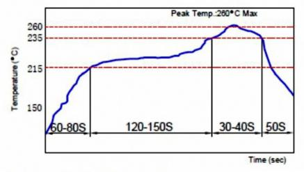
Preheating: 215°C for 120-150 seconds Soldering Temperature: 235°C for 30-40 seconds Peak Soldering Temperature: 260°C max for 10 seconds
